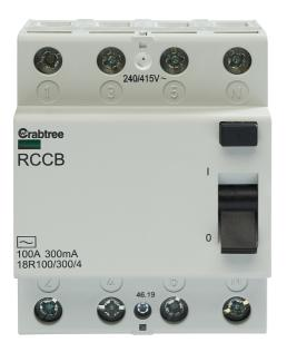
Four Pole RCCB, 100A 300mA, Type AC, For use with Crabtree Loadstar distribution boards, For incoming options can be used with 18LK125 connection kit
