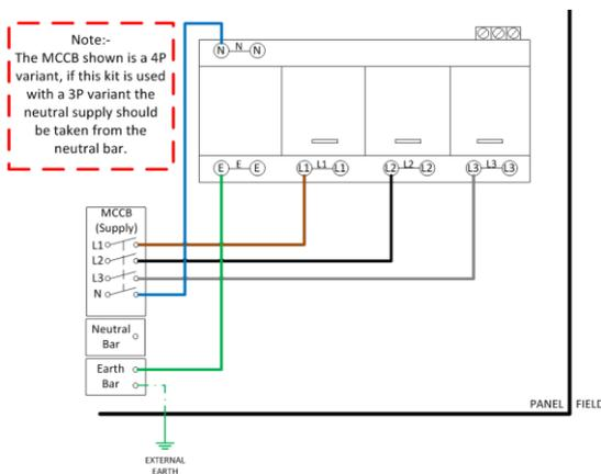
**Fig. 2 A - Lightning & Combination Arrestor Wiring Details**
