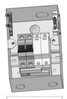
**Important Note:** Incoming cables must only be fitted into the top of the switch as shown
