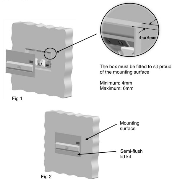
The consumer unit must be de-rated as follows: - Max. 100% rating, continuous load (in excess of 1 hour) 90% of incomer rating. The product number of the consumer unit on to which the kit is fitted must be recorded on the silver specification label affixed to the front cover.
