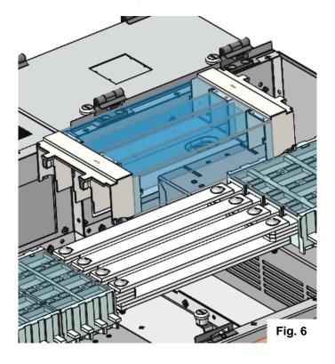
After the Add-On unit has been attached and busbar links and shrouds have all been fitted, all covers, gland plates and doors need to be refitted. The gland plates originally fitted to the panelboard are to be re-used on the Add-On unit, refer to Fig.7 for details.
