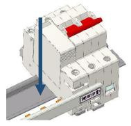
With the terminal cage of the SPD wound fully out, clip onto the DIN rail adjacent to the Isolator (Way 1.) If the busbar is already fitted it may need to be removed and re-fitted. Fully screw down the Live terminal using the appropriate tightening torque.
