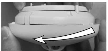
Figure 6 – Push Back the snap lock and turn the Alarm anti-clockwise
