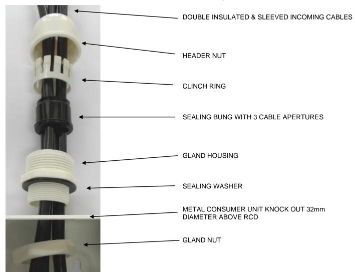
The kit comprises a 32mm insulated cable restraining gland, which is fitted by removing the knockout above the incoming terminals and fixing into position with the nut included. The incoming supply cables must be passed through the 3 aperture sealing bung. The sequence of assembly over cables is as shown above. Tighten the gland and header nut when installation of incoming cables is complete.
