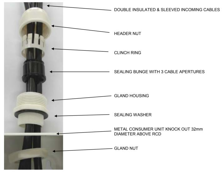
The kit comprises a 32mm insulated cable restraining gland, which is fitted by removing the knockout above the incoming terminals and fixing into position with the nut included. The incoming supply cables must be passed through the 3 aperture sealing bung The sequence of assembly over cables is as shown above. Tighten the gland and header nut when installation of incoming cables is complete. If the incoming supply cables are to be protected by conduit this must be of the all insulated type.
