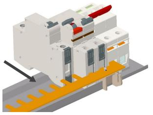
Locate device under edge of mounting plate and Slide onto busbar
