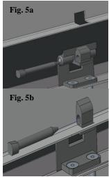
Secondly, place the pin into the hinge to secure the door in place. Ensure the pin is pointing downwards when fitting. Repeat this for all hinges
