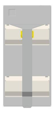
c) Now that the bracket is in position, depending on the diameter of the padlock shackle to be used, slide the U-Shaped locking bracket (with the correct hole in the tab) under the lip of the lid and through the cut-out in the T-shaped locking bracket.
