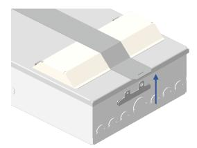
d) Hold both brackets in position and insert the padlock shackle through the hole in the bracket and lock shut.
