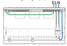
Fig 1 Incoming Terminal Connections
