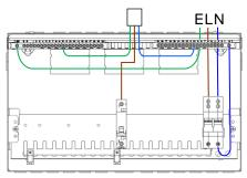
Fig 3.1 Connections to MCB's
