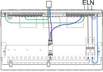
Fig 3.2 Connections to RCBO's
