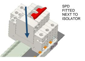
With the terminal cage of the SPD wound fully out, clip onto the DIN rail adjacent to the Switch (Way 1.) If the busbar is already fitted it may need to be removed and re-fitted. Fully screw down the Live terminal using the appropriate tightening torque.
