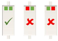
A full green window indicates a cartridge in good working order. Any red indication in the window means the cartridge is no longer working and must be replaced at the earliest opportunity.
