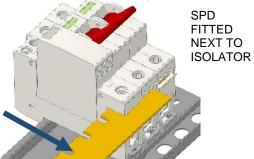
With the terminal cage of the SPD wound fully out, slide onto the busbar adjacent to the Switch (Way 1), ensuring that the busbar is underneath the screw head. Fully screw down the Live terminal using the appropriate tightening torque.
