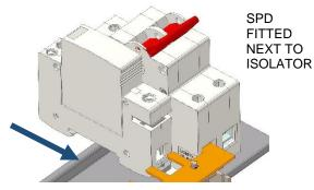
With the terminal cage of the SPD wound fully out, slide onto the busbar adjacent to the Switch (Way 1.) Fully screw down the Live terminal using the appropriate tightening torque.
