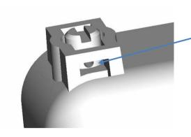
Insert wire or plastic seal through tamper-proof screw.
