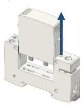
Remove the enclosure or consumer unit lid, slide the cartridge upwards from the base. Discard used cartridge in accordance with WEEE regulations.
