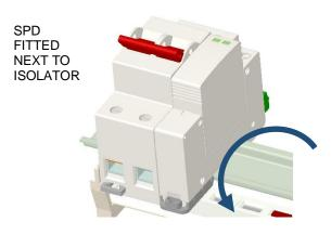
Place the SPD onto the top of the DIN rail and rotate to insert the prod into the busbar. The SPD should be fitted adjacent to the Isolator (Way 1.)
