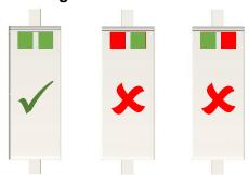
A full green window indicates a cartridge in good working order. Any red indication in the window means the cartridge is no longer working and must be replaced at the earliest opportunity.
